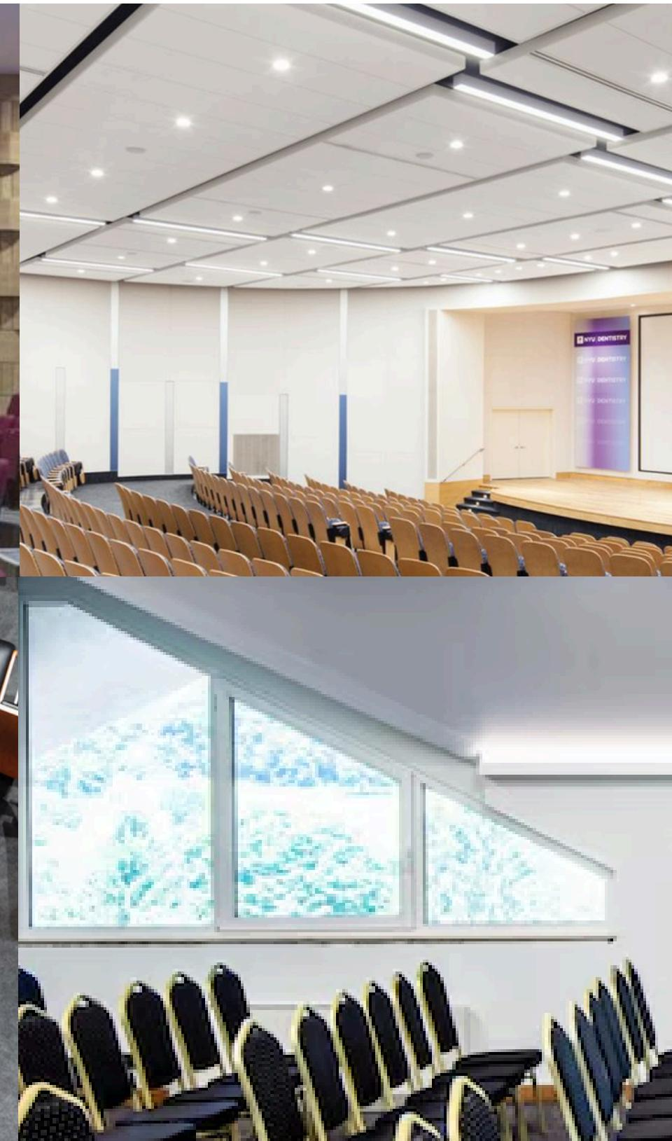
**Ceiling Systems:** Suspended acoustic tiles that control reverberation time
